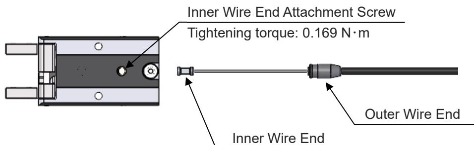
2. Confirm that the inner wire end is firmly inserted till the end of the hole. The position where the recess at the center of the inner wire end matches with the hole for the set screw should be the right position. With the inner wire end inserted to the end, tighten up the inner wire end attachment screw.
