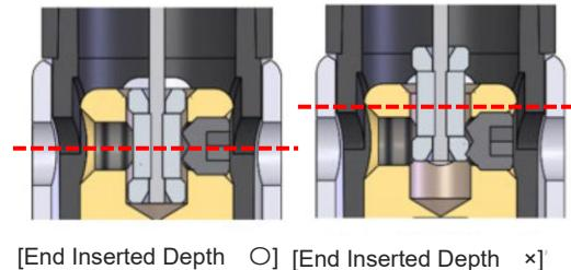
4. Insert the outer wire end till it reaches the end of the hole on the port. Tighten up the outer wire end attachment screw.
