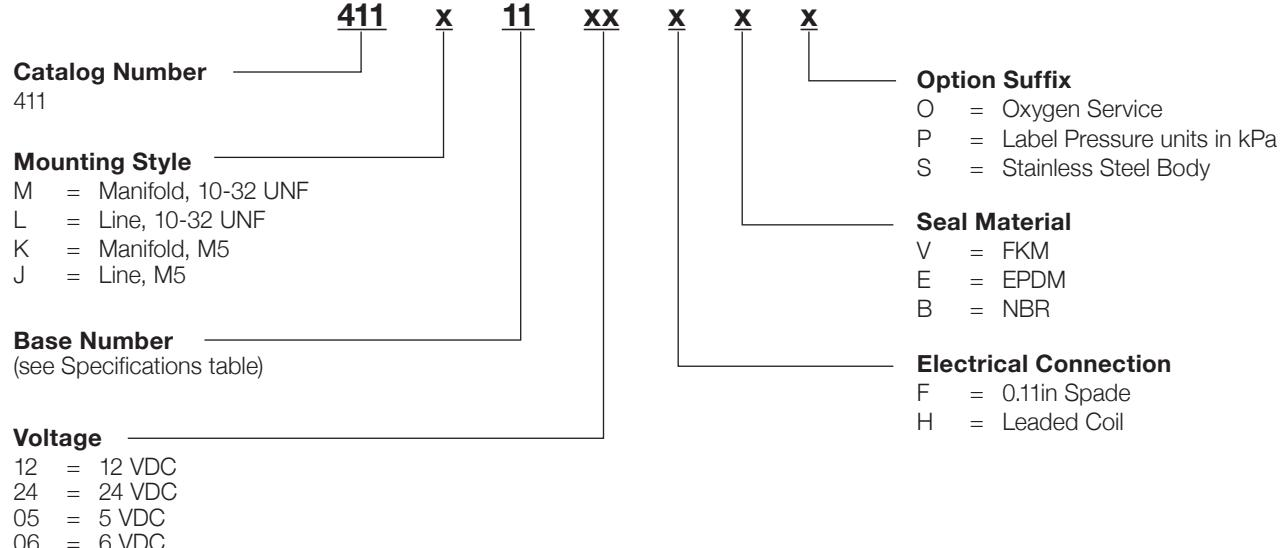
**NOTE:** Oxygen Service valves available with FKM or EPDM Seals only. UL / CSA available with 300 Series Stainless Steel Body. 3-Way Universal operation only available with leaded coil electrical connection (H).
