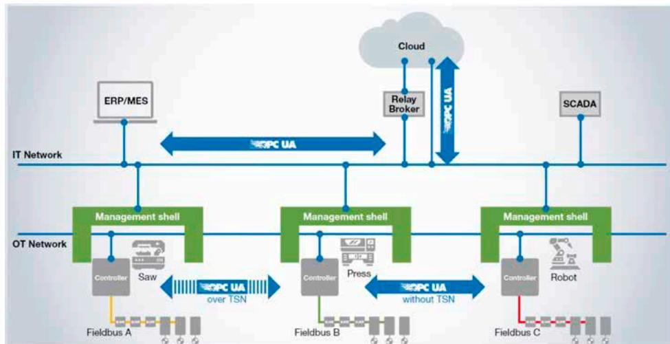
OPC-Unified Architecture (OPC-UA) is the innovative data exchange standard of the OPC Foundation. It ensures secure, reliable, and both manufacturer and platform-independent transfer of information that is not restricted or tied to any proprietary technology or manufacturer. OPC-UA allows access to any authorized application and to retrieve any information from anywhere and at any time.
