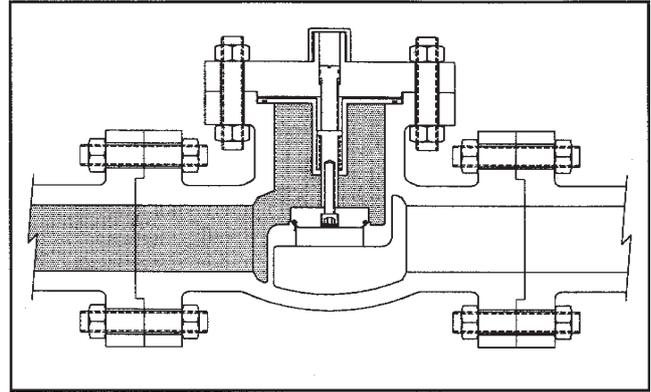
Valve Tripped Flow Shut Off
