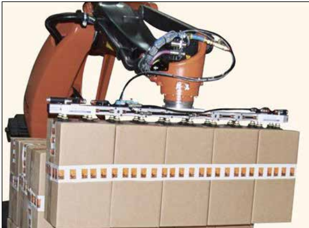
Vaccon designed, assembled, tested and shipped this new EOAT tool for a Kuka Robot in one day.
