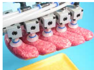
Multi-port pump EOAT with multiple manifold blocks and cups for food packaging operation.
