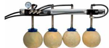
VP80-200H-MP and VP20-100H EOAT handle melons in fruit packing plant.
