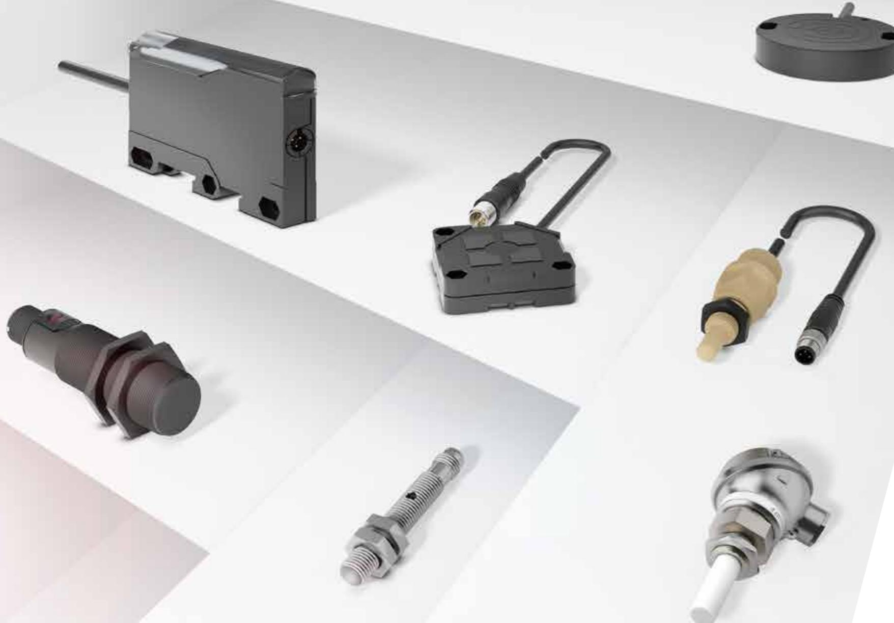
Balluff's capacitive sensors detect fluids, granulates and powders in direct contact or through a non-metallic container wall. Adhesive versions fit flexibly to the housing shape and are easily removable. Moisture, foam and deposits of any kind are compensated for, even through glass and plastic walls up to 10 mm thick. This makes them ideal as level detection sensors for conductive media while guaranteeing high application security.
