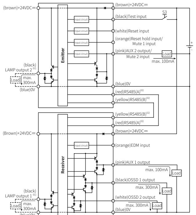
01) This wiring is used to activated the lamp output and displays the status to the external indicator based on selected output mode.
