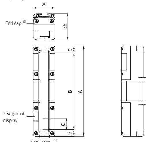
①) When removing the end cap, there is the lamp output terminal (top) or the power supply terminal (bottom).
